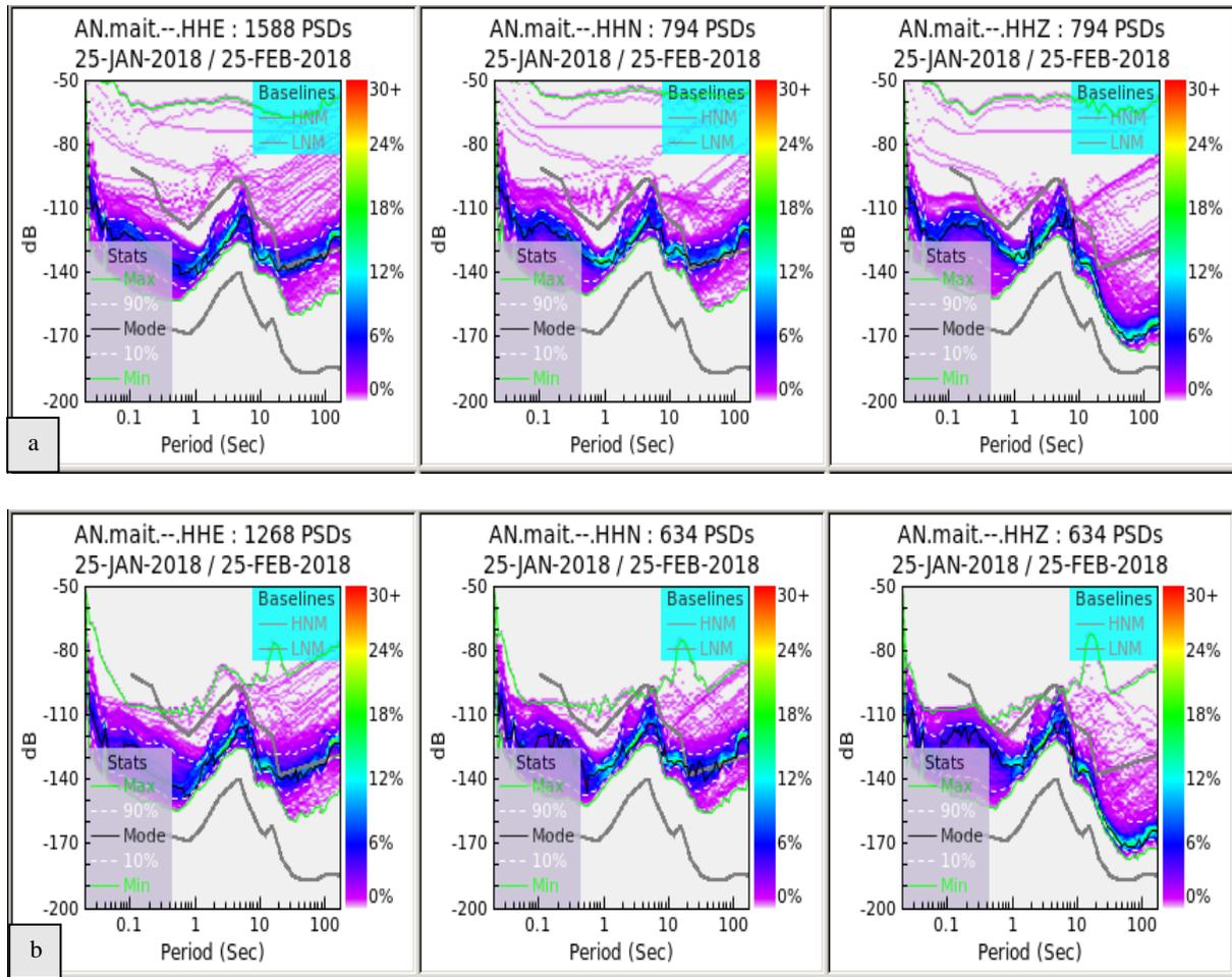
**Figure 6:** Power Spectral Density and Probability Density Function of Maitri broadband seismic station correspond to all three components HHE, HHN and HHZ (a) summer period day hours (b) summer period night hours.
