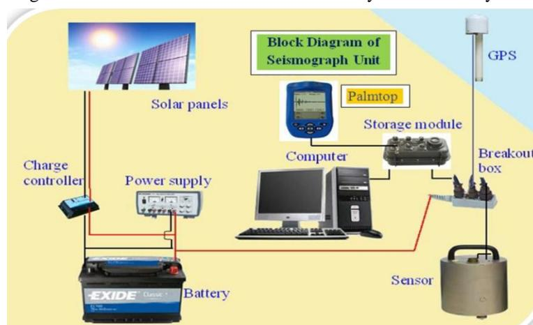
**Figure 2:** Block diagram of Seismograph setup at Maitri Station
